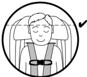
5. The harness straps must be in the closest position at or above the child's shoulders when seated.
