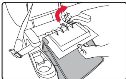
3. Turn and push the buckle retainer through the slot in the child seat shell.
