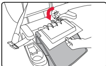
5. Remove the harness straps from behind the side wing covers.
