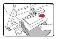
9 Unhook the clips at the front of the seat cover from the child seat shell, then remove the seat cover.
