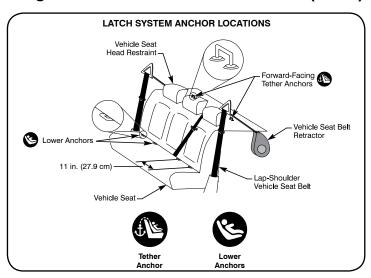
The Lower Anchors and Tethers for Children or LATCH, is a system available on this child seat that offers an alternative to vehicle seat belt installation methods. The figure above shows typical locations for lower anchors and tether anchors in a vehicle. See pages 2-3 for LATCH components on this child seat.
