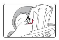
8 Attach the hook and loop fasteners on the head restraint cover around the harness.
