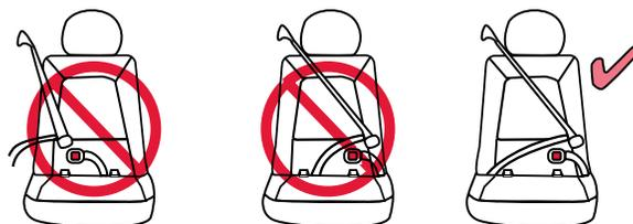
The vehicle belt fits properly when the lap part sits low across the child's upper thighs (b) and the shoulder part lies across the center of the child's chest and does not contact the child's neck when routed through the upper belt guide (a).
